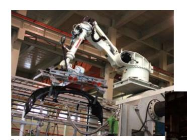
Releasing work from resin molding machine
